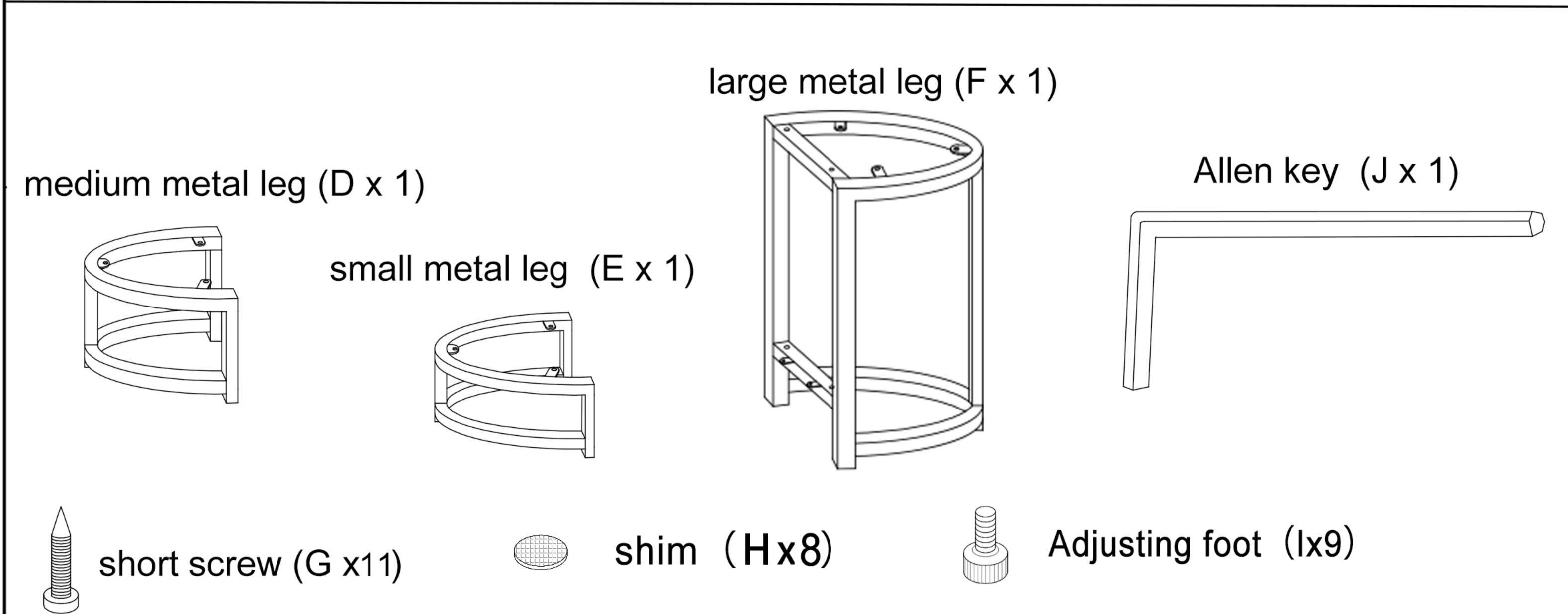
**Note:** Do not fully tighten all bolts until all parts are in place. Failure to follow these instructions may cause the bolt to misalign during assembly.
