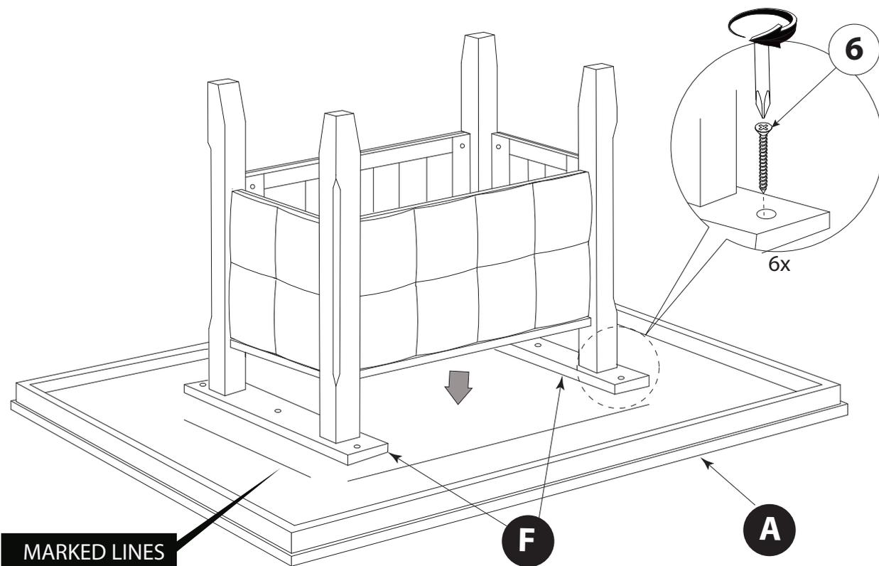
Turn the TABLE BASE upside down, attach the mounting bars to the underside of the TABLE TOP within the marked lines, align screws, and tighten them. Make sure all screws are fully tightened before turning the table table upright, by two adults or more.
