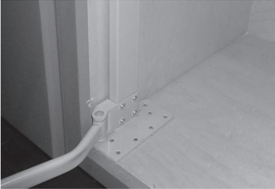
Firmly secure the Center Support on the open side of cabinet using (10) #6 x 3/4" flat head Philips wood screws.
