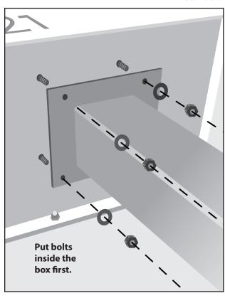
1. Attach the box to the pole with the four included 7/16" bolts, washers and nuts using your 7/16" Socket or Crescent Wrench.
