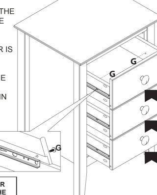
PUSH THE SCREW THROUGH THE DRAWER SIDE FROM THE INSIDE OF THE DRAWER INTO THE DRAWER RUNNER AND SECURE.
