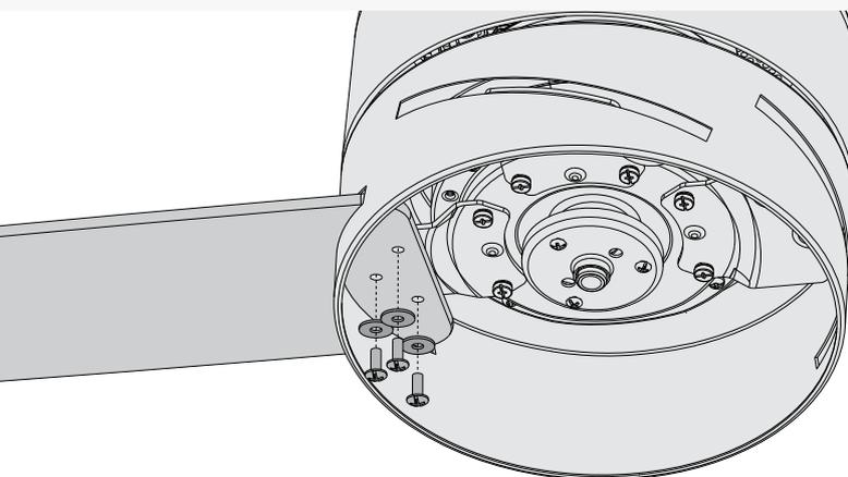
Put the blade washers found in the ■ hardware bag onto the blade screws found in the ▲ hardware bag. Then install the blade screws to secure each blade to the fan.
