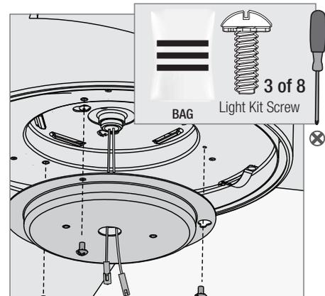
Feed the light wires through the hole in the lower switch housing. Align the lower switch housing screw holes with the bottom of the light kit assembly. Using the three light kit screws, found in the hardware bag, mount the lower switch housing to the light kit.
