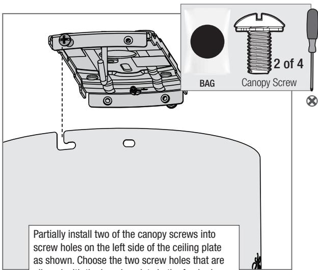
Partially install two of the canopy screws into screw holes on the left side of the ceiling plate as shown. Choose the two screw holes that are aligned with the hanging slots in the fan body.
