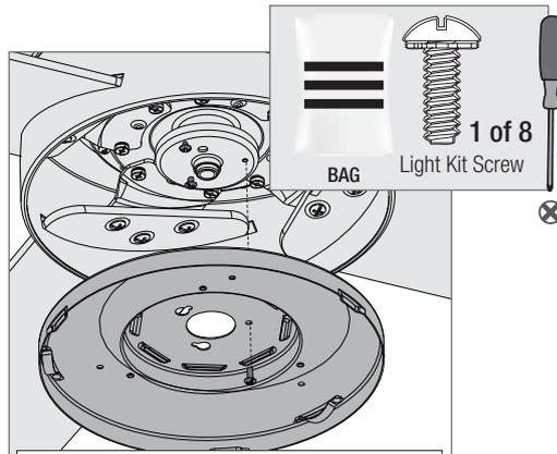
Align the keyhole slots in the top of the light kit assembly with the partially installed assembly screws. Rotate the keyhole slots around the screws and twist counterclockwise. Tighten all three screws securely.
