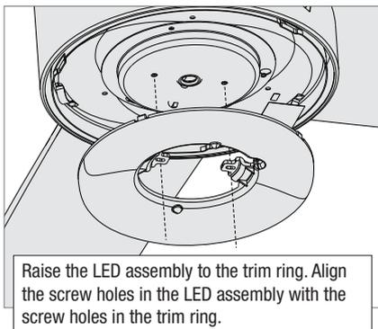
Raise the LED assembly to the trim ring. Align the screw holes in the LED assembly with the screw holes in the trim ring.
