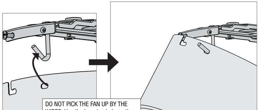
**DO NOT PICK THE FAN UP BY THE WIRES.** Use the hanging hole on the body of the fan to hang the fan on the hook of the ceiling mounting plate.
