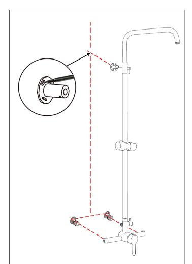
**6.** Hold the assembled shower set in its desired position and mark the location of the mounting bracket.
