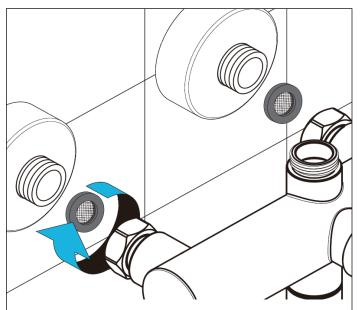
**10.** Connect the main body to the installation adapters. Make sure to use sealing washers.
