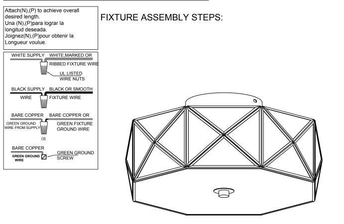
110-120V / 60Hz E26 4\*MAX 60W TYPE A (Do not contain light bulb)
