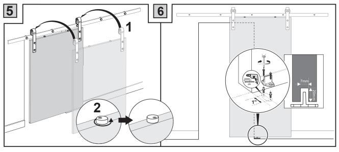
Attach the door to the rails making sure that the anti-jump disks are engaged to avoid a serious accident.
