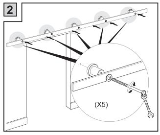
Attach the rail to the wall brackets using a wrench to fasten
