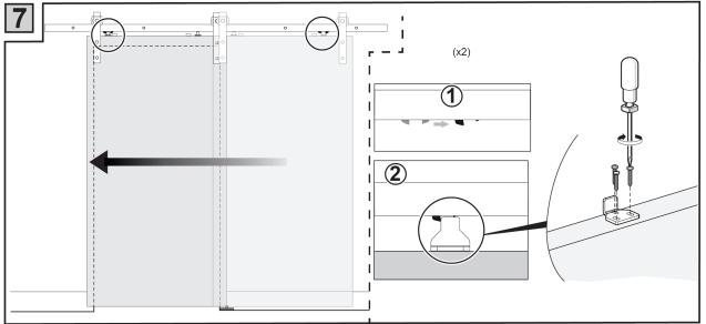
Set the catches on the soft-closing mechanism to the open position. To determine the positioning of the soft-close triggers, it is recommended that the doors be moved to the fully open position. Determine where the soft-close trigger would engage the soft-close mechanism and mark your drill holes on the top of the door. Move the door to the fully closed position and repeat to determine the placement of the second soft-close trigger.
