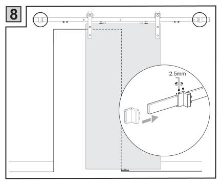
Adjust the door stops accordingly using the provided 2.5mm Allen key.
