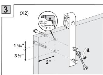
Drill out holes in the door using a 10mm routing drill bit as pictured. The bottom of the doors should be routed at this time in order to accept the floor guide.
