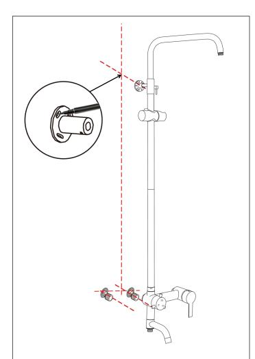
**6.** Hold the assembled shower set in its desired position and mark the location of the mounting bracket.
