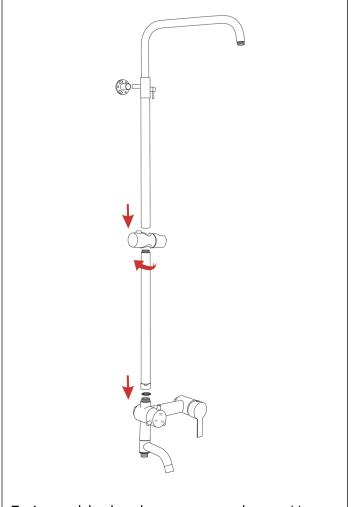
**5.** Assemble the shower set as shown. Use sealing washers where needed.
