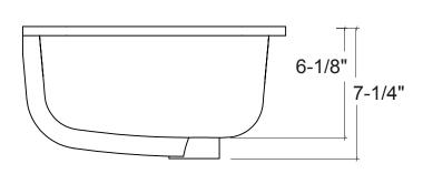
By IAPMO, ceramic lavatory warpage is defective only if warpage of flat slab out of horizontal plane exceeds 6.3 mm/m (0.25 in/ft) on all sizes
