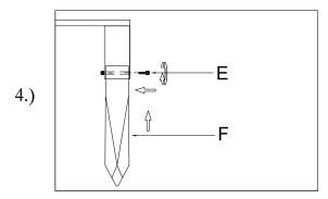
Step 4: Attach glass (F) using set screws (E).
