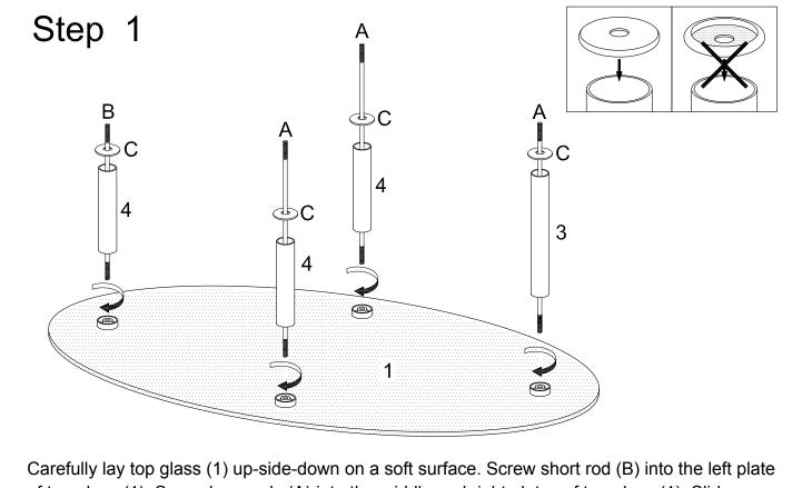
of top glass (1). Screw long rods (A) into the middle and right plates of top glass (1). Slide cylinders (4) onto short rod (B) and middle long rods (A). Slide cylinder (3) onto right long rod (A). Slide decorative rings (C) onto rods (A, B) and snap onto cylinder (3, 4).
