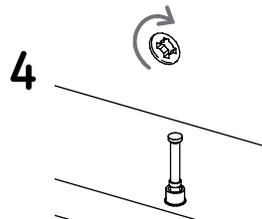
After joining two panels together you should turn the cams 180° with a phillips head screwdriver to adjust and secure the joint.
