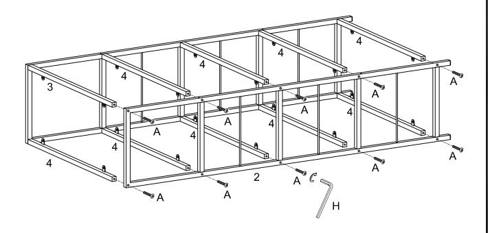
Attach supports (4) to legs (2) using bolts (A) as shown.
