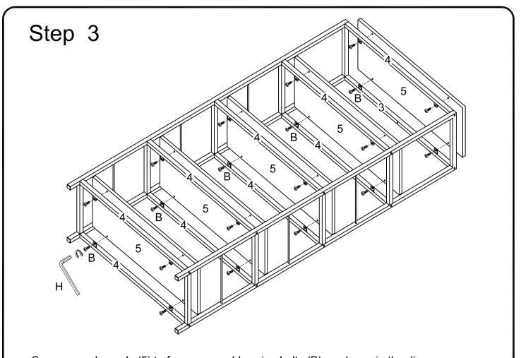
Secure wood panels (5) to frame assembly using bolts (B) as shown in the diagram.
