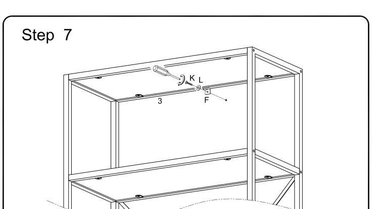
(Optional) Secure unit to the wall using screws (K) and washers (L) at the installation points of wall plugs (J) from previous step.
