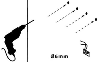
For drywall installation, mark the hole locations and drill  $\Phi$  6mm holes for the drywall anchors. Install a junction box behind the mirror for power connections.
