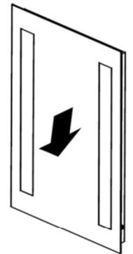
Press the mirror down slightly and make sure the brackets fit properly.
