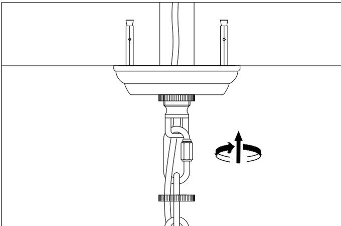
3. Slide the canopy over the ceiling plate. Hang the lamp from the suspension eye, using the chain and carabiner. Carefully lower the lamp until the chain is taut. Straighten the chain links.
