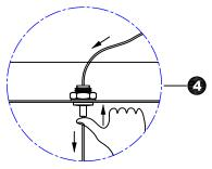
**Note:** Press the wire restraint to adjust the desired length of cable.
