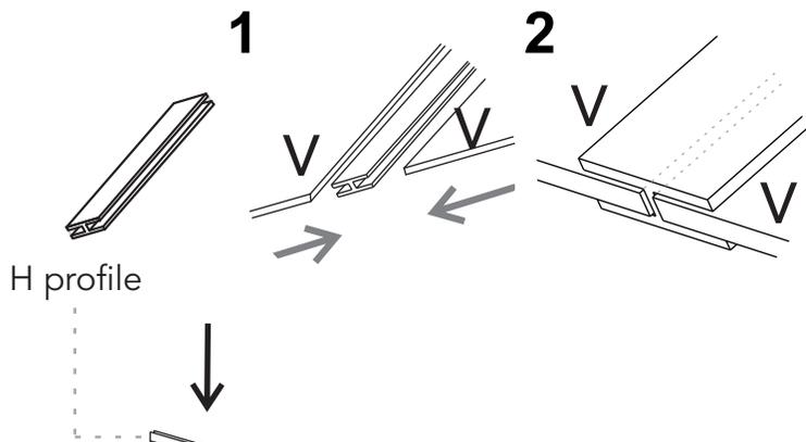
3 Slide the back panel inside the grooves.
