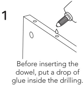
Before inserting the dowel, put a drop of glue inside the drilling.
