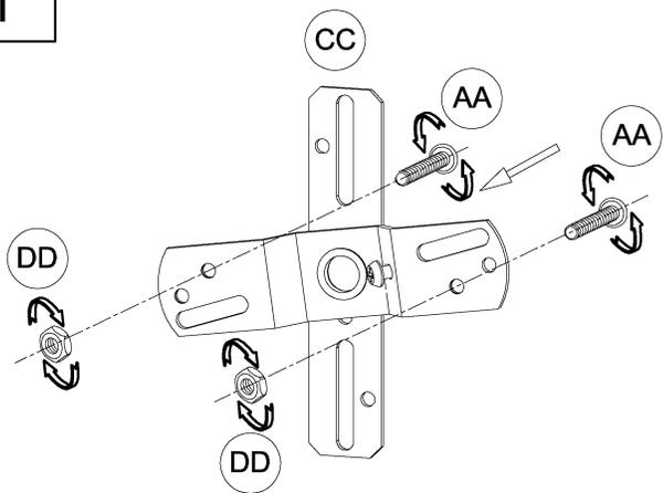
1. Screw screw (AA) onto swivel mounting strap (CC) and use hex nut (DD) to secure it tight.
