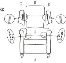
2. Place Bracket into Sleeve and press top of back down firmly to lock your KD back and KD wings in place Connect the connector of back and seat.
