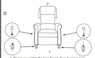
1. Please assemble the legs first before turning over the chair in order to avoid motor broken. Take down the bag from the bottom of the chair, legs are
