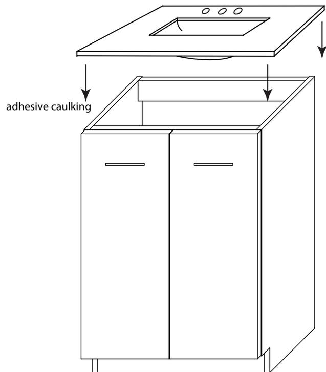
**Step 3 :** Secure top & back splash to cabinet by using adhesive caulk
