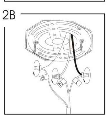
Strip 3/4" of insulation from wire ends. Connect house ground wire to fixture ground wire marked with symbol. Twist wires together using wire nut. Connect black house wire to the fixture wire marked "L". Twist wires together using wire nut. Connect white house wire to the fixture wire marked "N". Twist wires together using wire nut.
