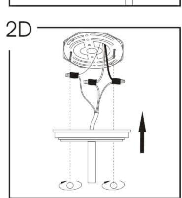
Lining up threads on mounting plate with holes in fixture canopy, attach fixture to junction box using cap nuts. Be sure to carefully tuck wires into canopy while attaching.
