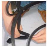
4. In turn, make all rings up and down assemble by bolts tightened with screwdriver.
