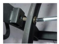
2. According to the same method above, assemble all stand legs but bolts cannot be twisted too tight.
