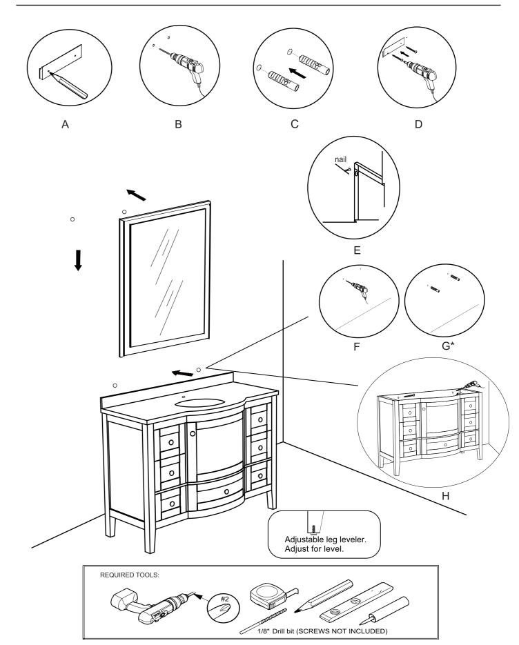
\*SECURE SCREW TO STUDS WHEN POSSIBLE
