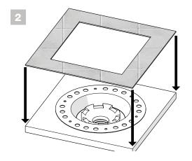
A. Install flooring surface, leaving a 6-1/2" opening to access Drain.
