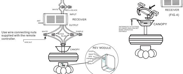
If other fans or supply wires are different color, have this unit installed by qualified licensed electrician.
