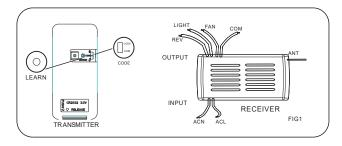
If there are two or more ceiling fans installed in the same house, in order to prevent your ceiling fans from being affected by the remote control of the adjacent ceiling fans, first turn the switch in each remote control transmitter to the CODE(locked) position (see the schematic diagram FIG1) Remarks: The standard state of the transmitter is in the common code COM.
