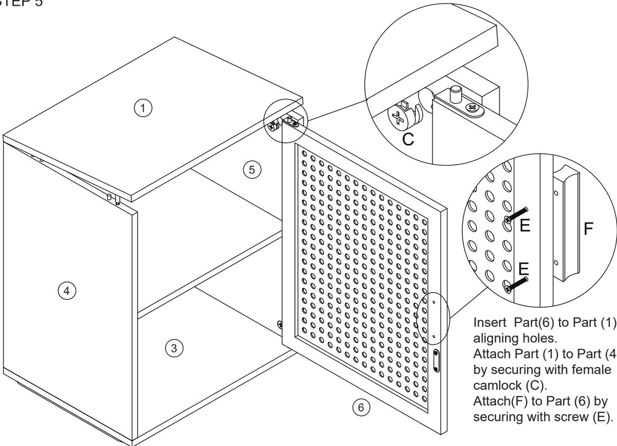
Insert Part(6) to Part (1)(3) by aligning holes.
