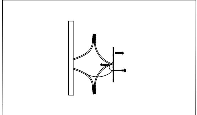
1. Remove mounting bracket from fixture and install to electrical box. Then wire fixture to wires in outlet box. Copper wire is for Ground.
