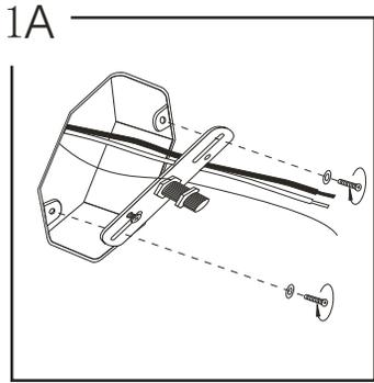
Carefully pull house wires out of junction box. With threads facing outward, screw crossbar into junction box using outlet box screws.
