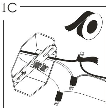
Tape wires and wire nuts together using electrical tape.
