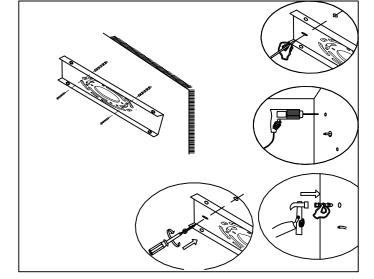
Step.1: Remove mounting bracket (A) from Canopy (C) to install to electrical box
