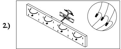
Step.2: Wire fixture to wires in outlet box. Green wire is for Ground.
