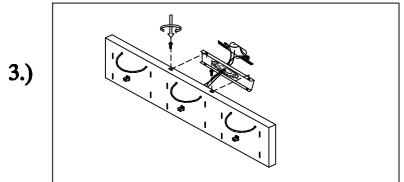
Step.3: Secure fixture to mounting bracket using screws (D).
