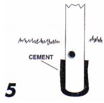
Place post at the center of the hole then fill with concrete to just below the wire inlet hole at the post base.
