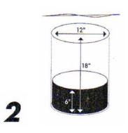
Dig a hole 12" diameter by 18" deep. Fill in 6" with gravel.
