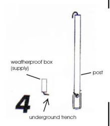
Make power connection through a weatherproof box and run line through trench to lamp post hole. Feed line from the inlet hole at post base to the top of the post.
