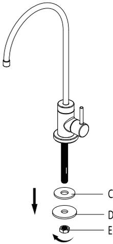
Remove the rubber washer (C), metal washer (D), and mounting nut (E) from the end of the stud.
