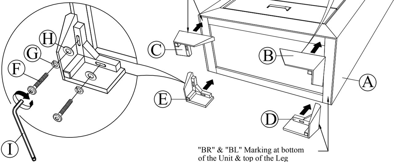
"BR" & "BL" Marking at bottom of the Unit & top of the Leg
