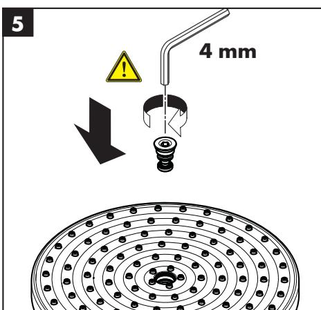
**!** Do not overtighten the air injector or damage may result.
