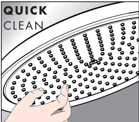
Remove scale deposits in the spray channels by rubbing across the channels using a finger or a sponge.
