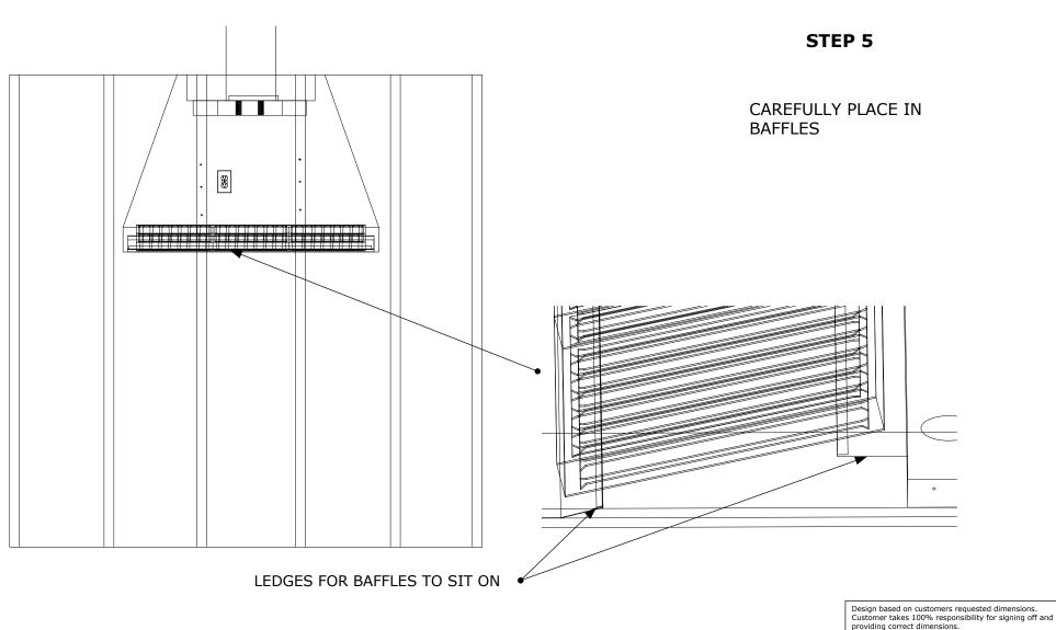
DESCRIPTION: SCALE: SHEET: DATE: REV: N/A 02/08/18 5/5 INSTALLATION GUIDE (REAR DUCTING BY: DE TOLERANCE: +/- 1/8" JOB: LOCATION) ... NAME SIGNATURE DATE
