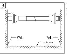
3. Holding the larger sized rod, rotate the smaller rod until it is locked into position securely.
