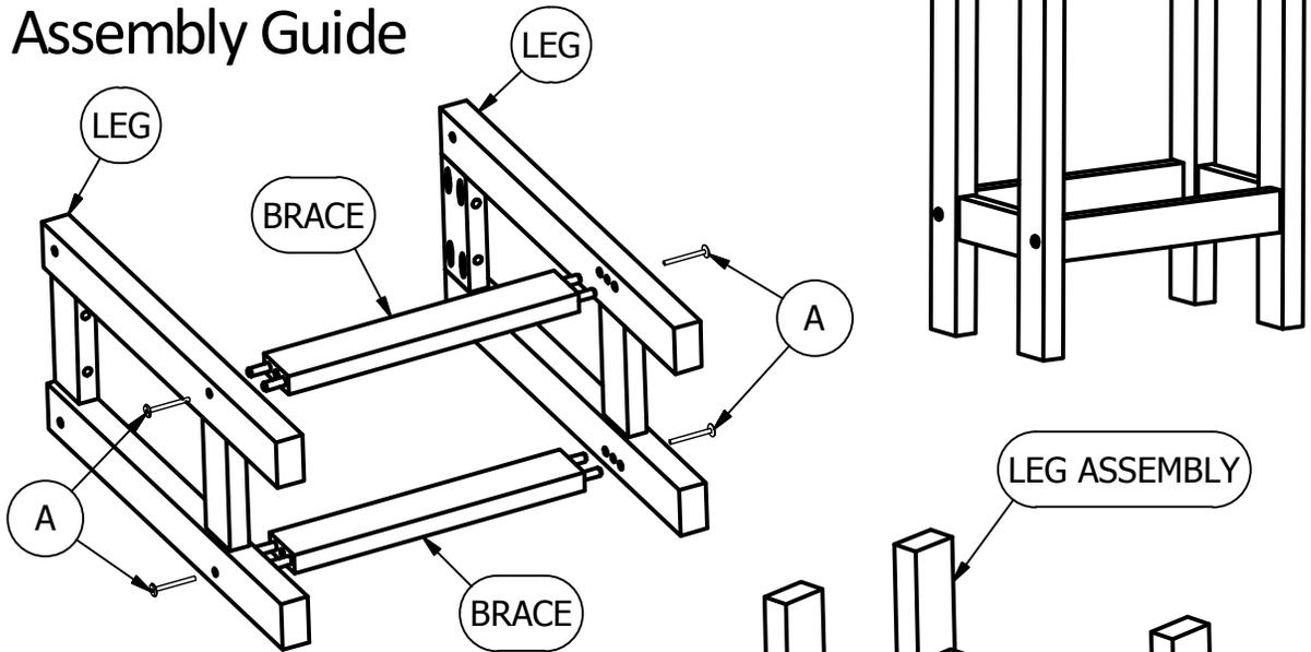
**1)** Install Braces Between Legs Using (4) "A" Bolts as Shown.
