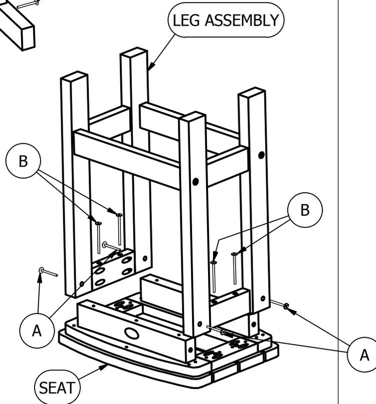
**2)** Attach Leg Assembly to Seat Using (4) "A" Bolts and (4) "B" Bolts as Shown.
