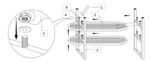
Step 1: Turn iron leg (3) upside down to assemble the shelf (2). Fasten the shelf with iron leg by round washer (A) and nut (B). Note: Do not screw too tight until assemble the other side.
