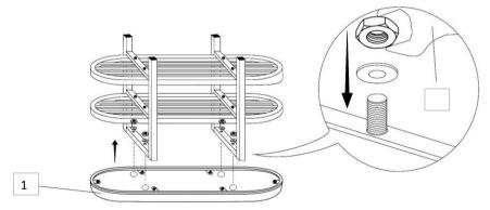
Step 2 : Insert the finshed iron frame to the downside bench top (1). Attached them by round washer (A) and nut (B), then screw by wrench (C).
