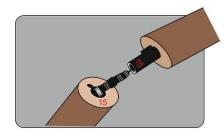
Screw the protective cap over the connectors to ensure a watertight seal.
