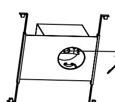
Screw adaptor into socket in recessed housing.
