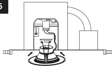
Gently squeeze together the torsion springs of the LED trim and insert into the recessed housing.
