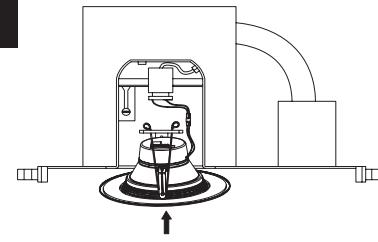
Gently push up the LED downlight until trim is flush with the ceiling. Ensure no wires are exposed. **Turn on power.**
