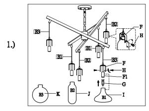
Step.4: Insert the G9 bulbs into socket one by one, Attached the glass(B1, B2, B3) to yoke(F), and secured with lock screw(H)
