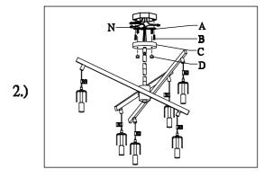
Step.3: Wire fixture to wires in outlet box.
