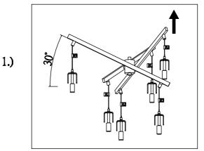
Step.1: Adjust the lamp body(F), adjust the tube to up 30 degree after remove package
