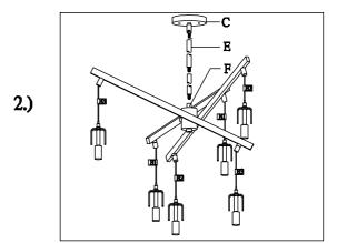
Step.2: Carefully remove packaging from fixture.Run wire through stems (E) and combine stem lengths to meet desired mounting height. Then attach canopy (C) to fixture.
