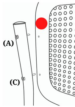
Please locate top of backrest and position the backrest facing up. You will see color codes on screw (A) which will match the color code on the back of the frame to verify the backrest is positioned correctly. Place the backrest against the frame, screw in the top hole first (A) and then the bottom hole (C). (Do not tighten the screws until both screws are in halfway).
