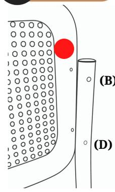
Once tightened move to the other side to attach the two remaining screws. First start with top (B) and then move to the bottom (D). Note: Assembly person no. 2 will need to help to pull/adjust and flex the top two metal back posts of chair frame towards each other as needed. Tighten all screws until the metal frame is touching the wood. (Caution : Do not over tighten screws)
