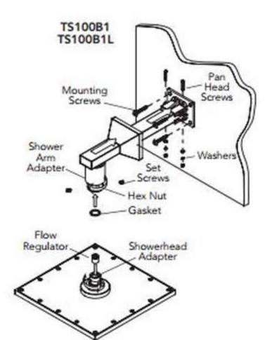
TOTO<sup>®</sup> logo is parallel to the wall (slightly loosen the showerhead if necessary), then tighten with set screws.
