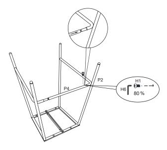
$Step \ 3. \ Insert \ ring(P4) \ to \ leg \ frame(P2\&P3) \ using \ bolts(H1) \ and \ 80\% \ tighten \ bolts \ with \ allen \ wrench(H6) \ as \ illustration \ below.$
