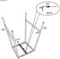
Step 2. Insert ring(P4) to leg frame(P2&P3) using bolts(H1) and 80% tighten bolts with allen wrench(H6) as illustration below.
