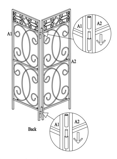
Attach Left Frame A2 to Right Frame A1 as shown above.
