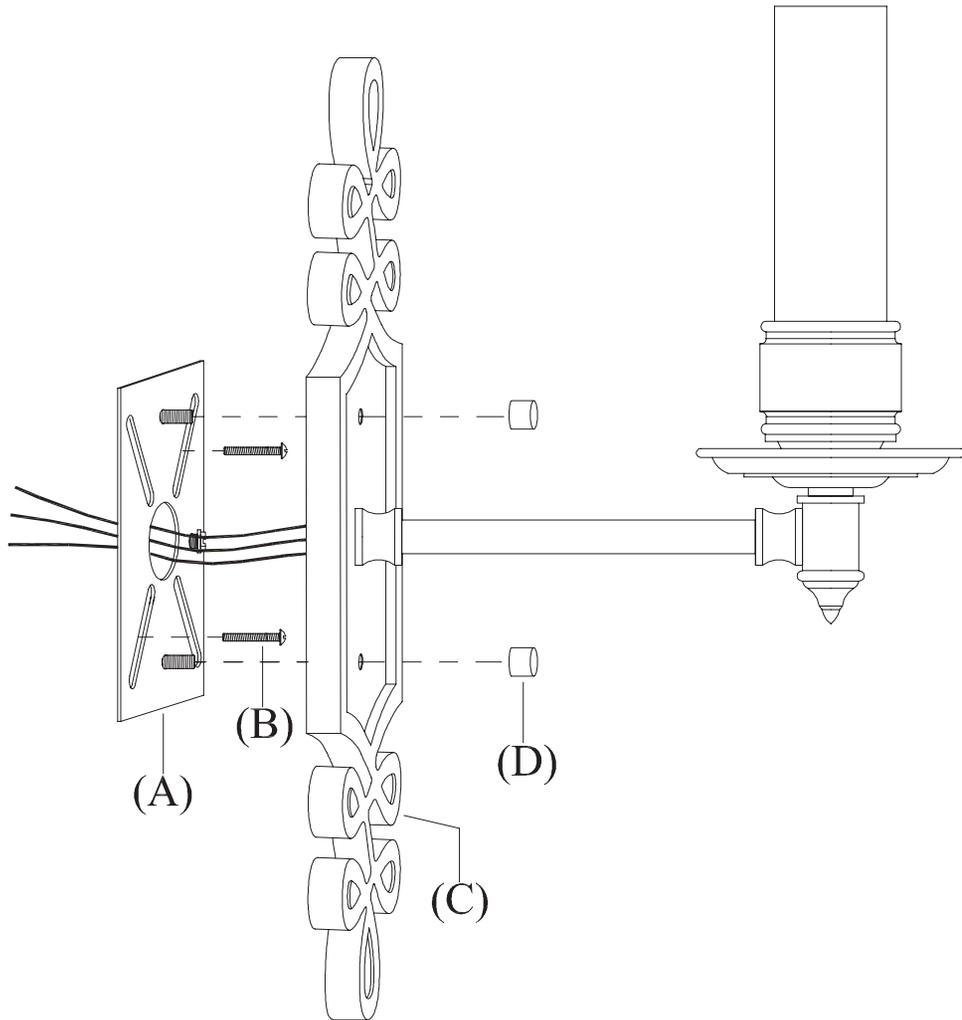
1. Attach ground (green) wire to ground wire from wall outlet box (usually green or copper in color), fasten together with a plastic wire connector. Tightly wrap the wire connector with electrical tape so the end of the connector is sealed. IT IS IMPERATIVE THAT THE OUTLET BOX IN YOUR HOME BE PROPERLY GROUNDED.
