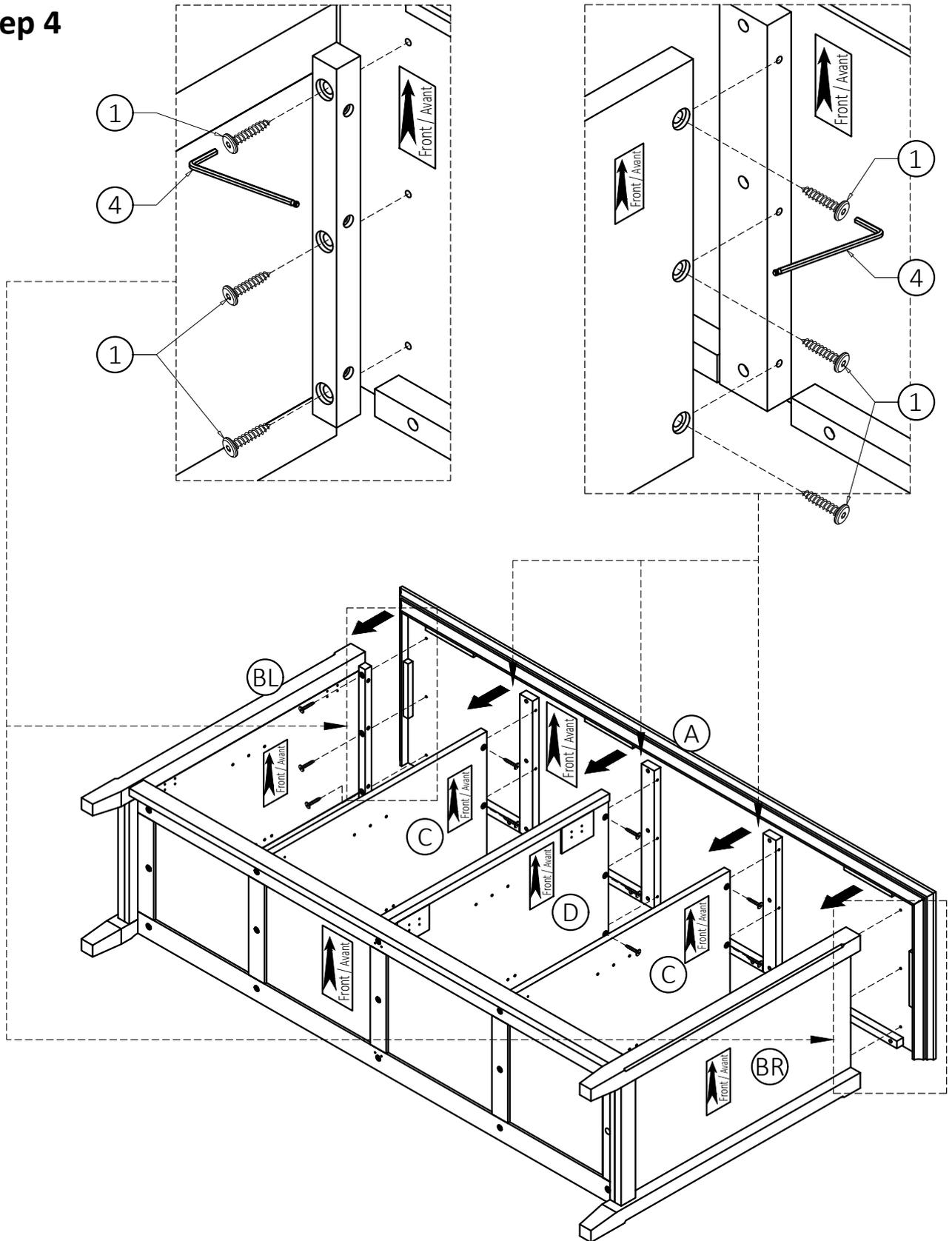
1. Use three Allen Key Screws ① to attach each part ②L, ②R, ③, ④ through guide holes each part ②L, ②R, ③, ④ to pre-drilled holes of Top ①.
