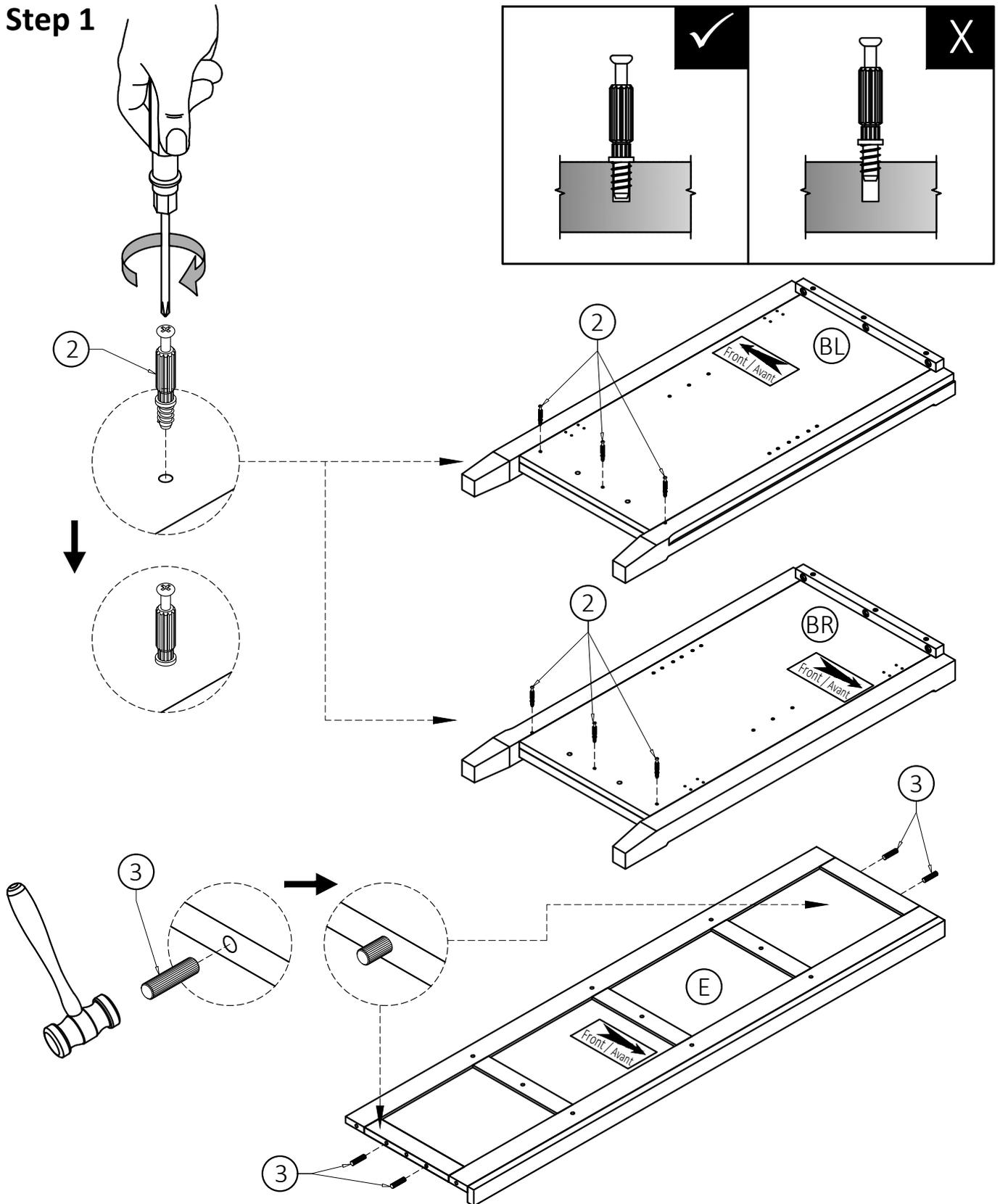
1. Attach three Cam Lock Pins ② into pre-drilled holes on each part (BL), (BR).
