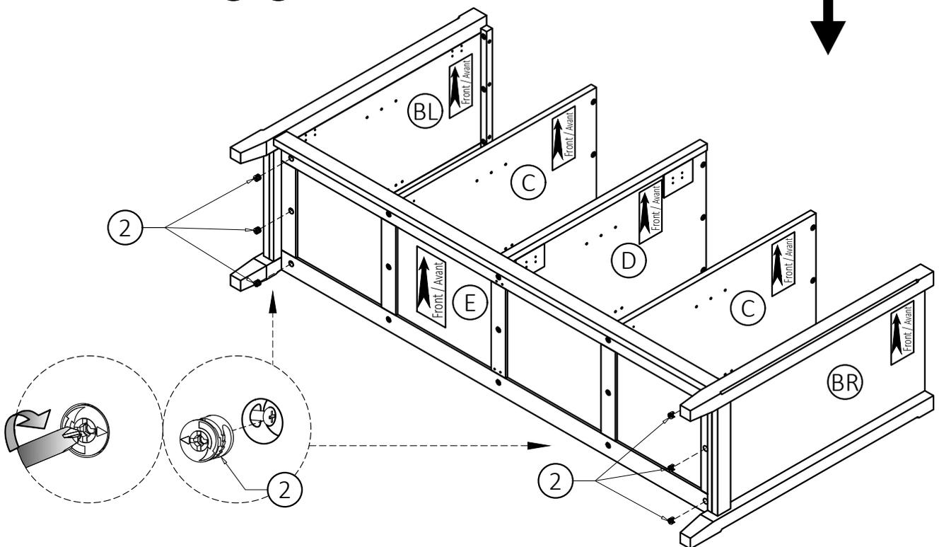
2. Insert six Cam Locks (2) into guide holes on part (E).
