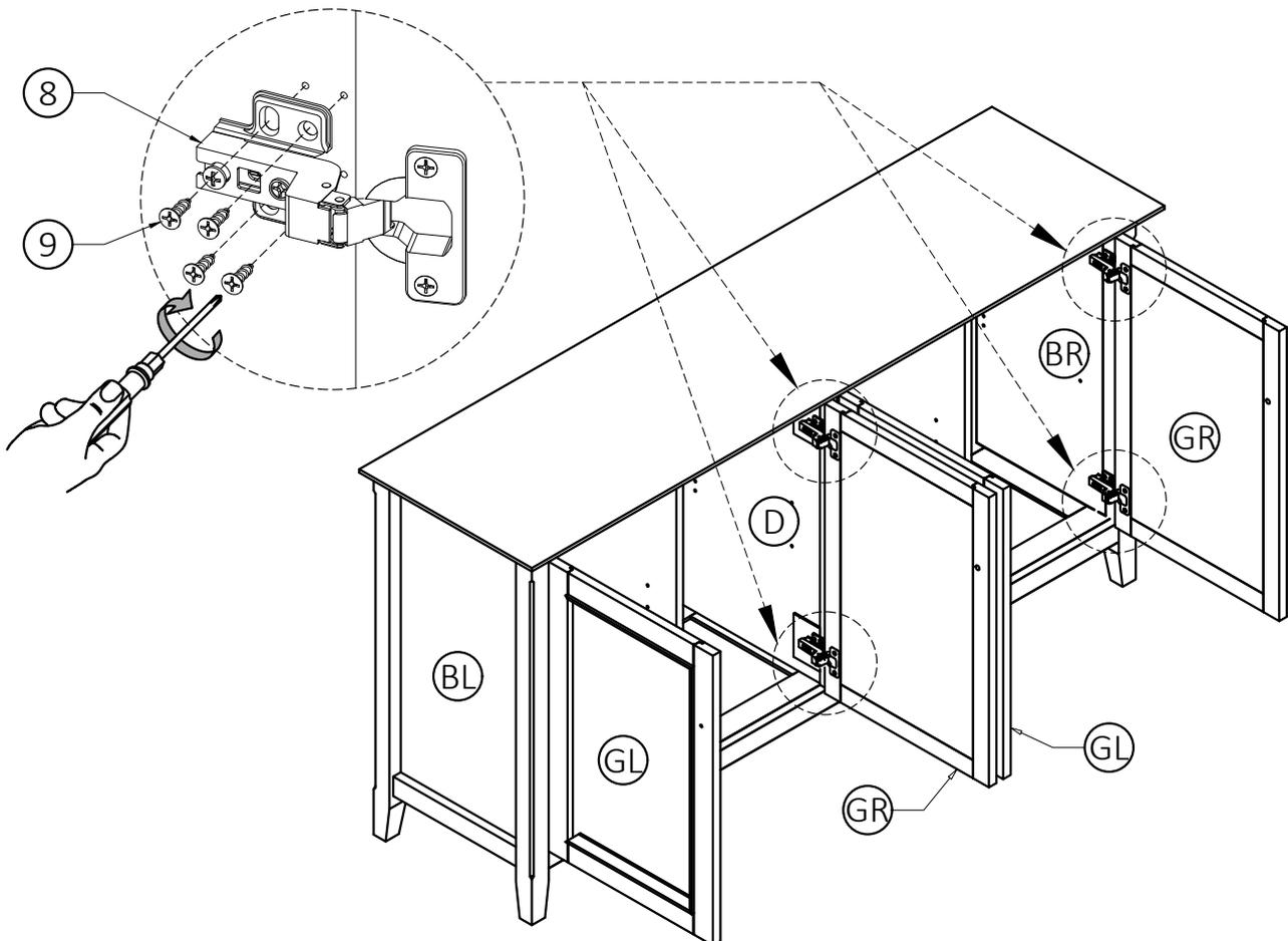
2. Attach Adjustable Hinges (8) on Doors (GL), (GR) to parts (BL), (BR), (D) using Phillips Screws (9) into pre-drilled holes on parts (BL), (BR), (D).
