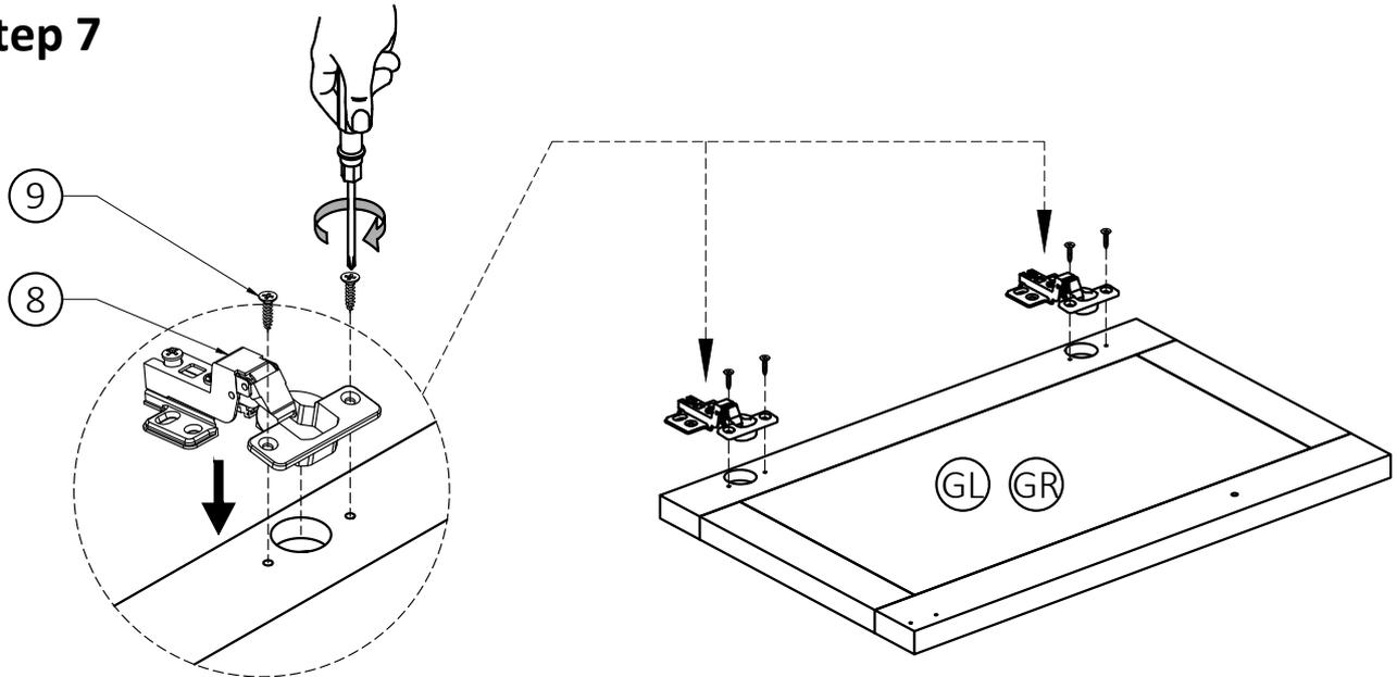
1. Attach Adjustable Hinges (8) to Doors (GL), (GR) using Phillips Screws (9) into pre-drilled holes on Doors (GL), (GR).
