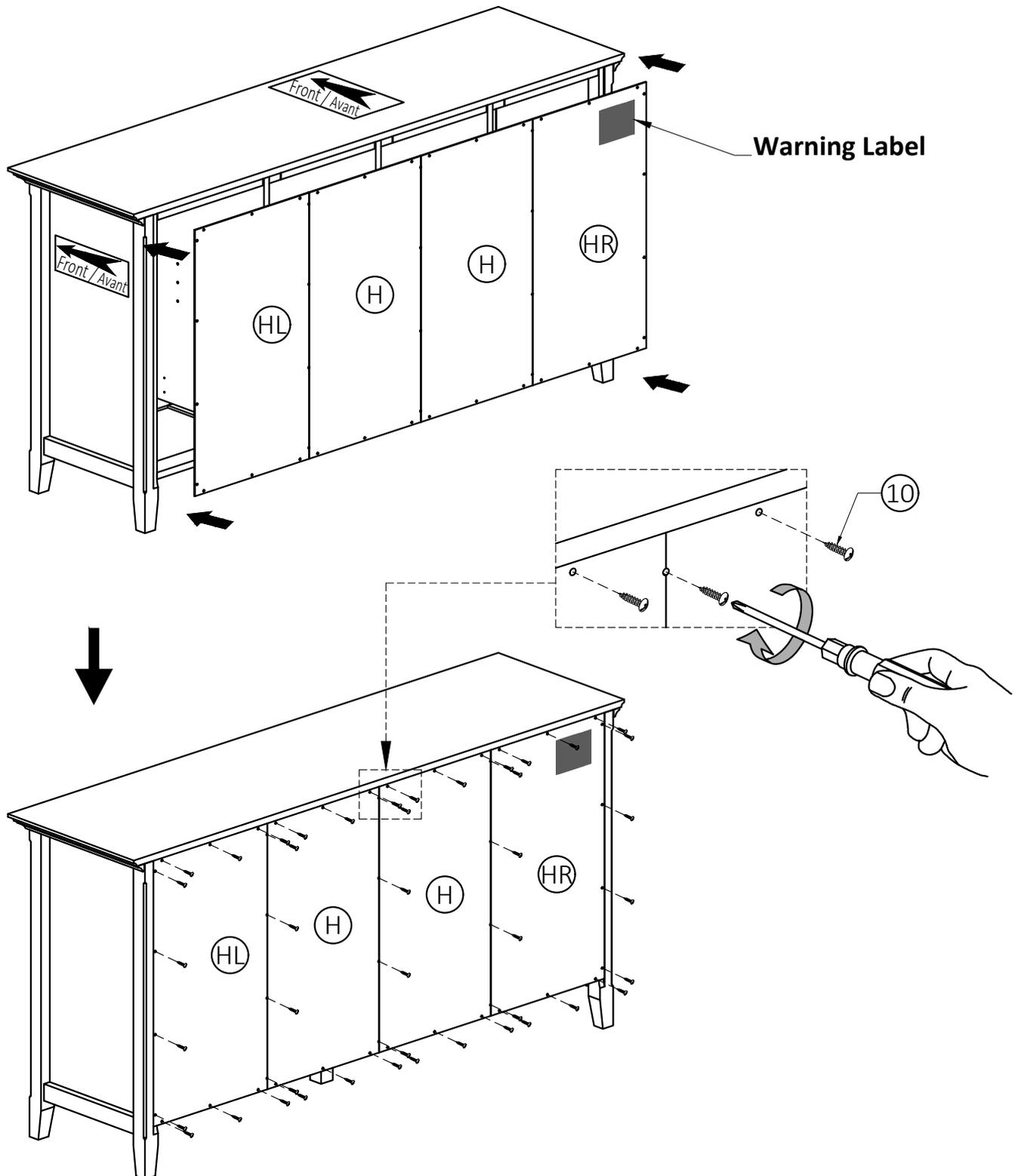
1. Attach the Back Panels (HL, HR, H) to back frame using Phillips Screws Round Head (10) through guide holes from Back Panels.
