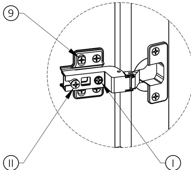
Tighten the Screw marked ⑪ to fasten hinge. The door may need to be adjusted so that all the spaces between the door and the unit sides are equal.
