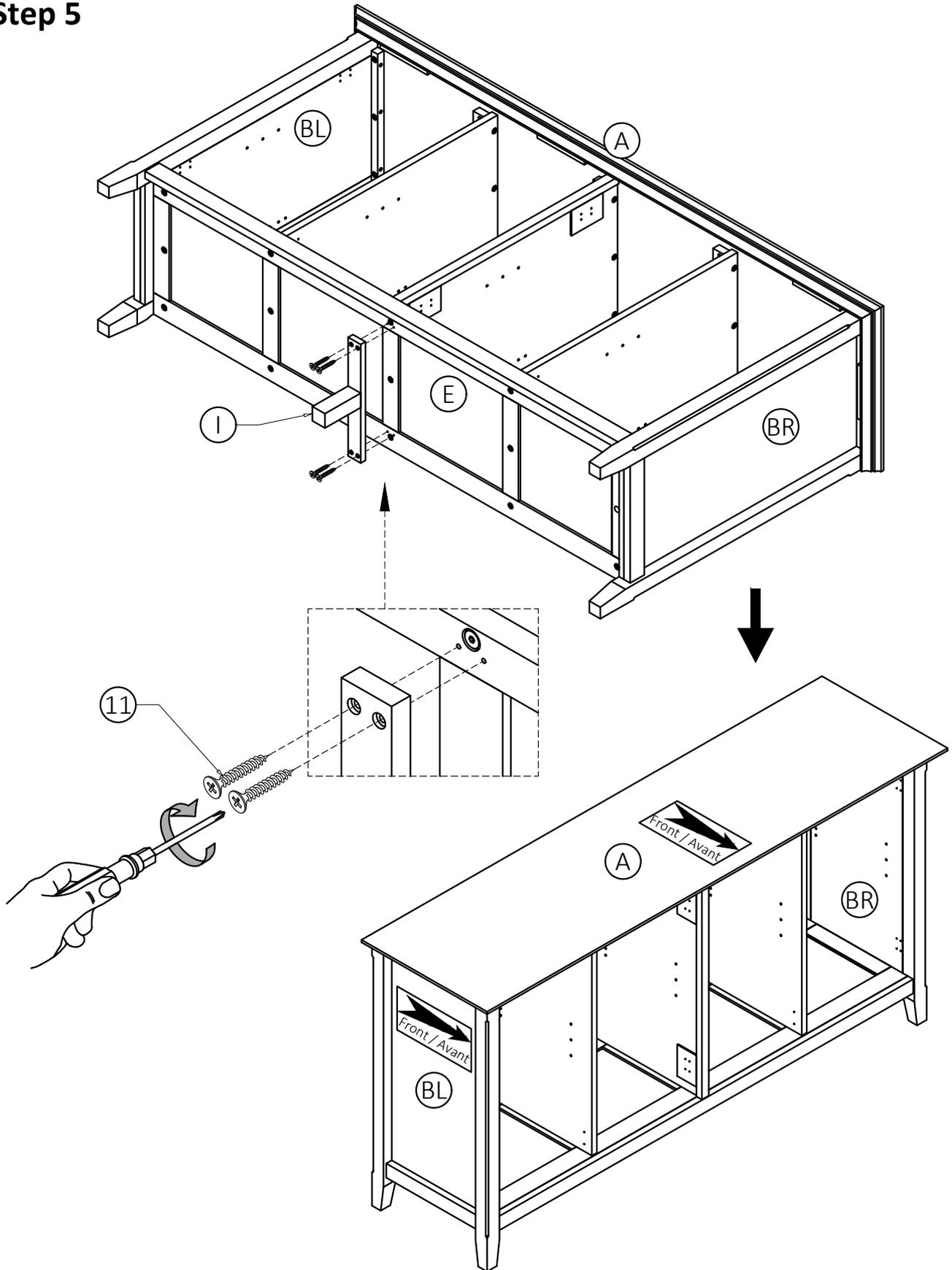
1. Align Bottom Support Leg (I) with pre-drilled holes on back of Bottom Shelf (E). Use Phillips Screwdriver to tighten four Phillips Screws (11).
