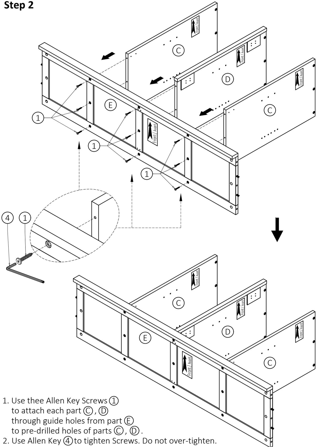
1. Use three Allen Key Screws ① to attach each part ③, ④ through guide holes from part ⑤ to pre-drilled holes of parts ③, ④.
