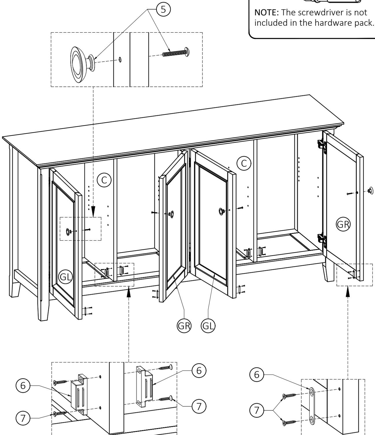
1. Attach Magnet Plates ⑥ to bottom corner of Doors ④L, ④R using Phillips Screws ⑦ into pre-drilled holes on Doors ④L, ④R.
