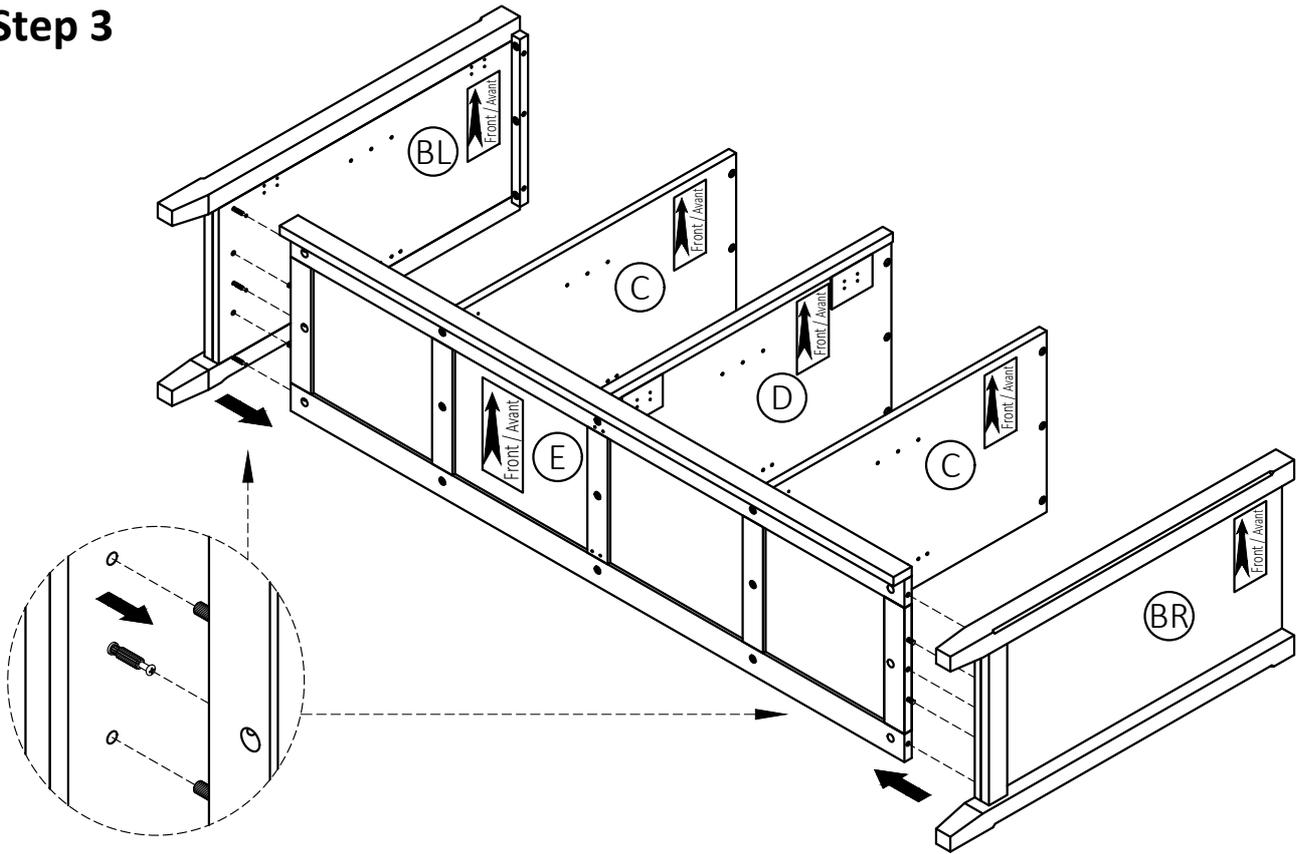
1. Align Cam Lock Pin and Wood Dowels with guide holes and attach parts (BL), (BR) to part (E).
