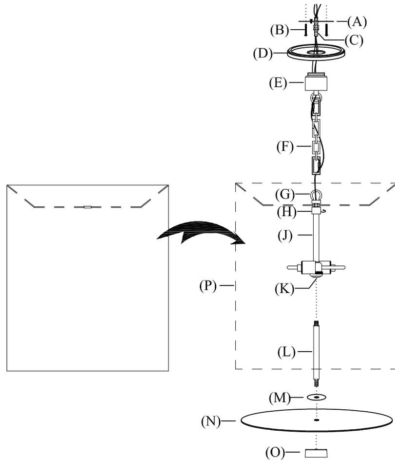
1. Attach chain (F) to top loop (G) on stem (J) by opening/closing end link of chain.
