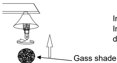
Install the glass on the lampholder, Do not over tighten.
