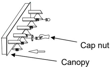
Attach the canopy to the mounting plate with screws provided.
